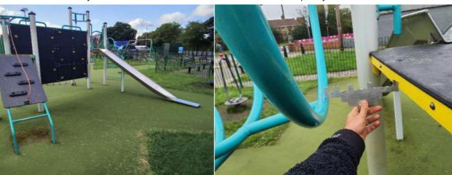
Finding: The item fails to meet the requirements of BS EN Action: Monitor - No remedial work recommended 1176 Part 1 4.2.7.2 for head and neck entrapment in the framework
