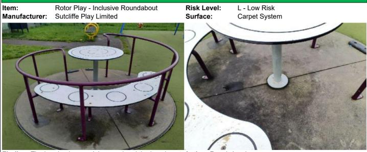
**Finding:** The bearing is worn / damaged and the item is not **Action:** Repair / replace operating correctly
