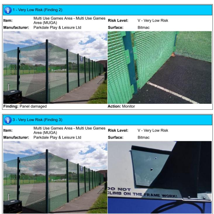
Finding: 2 nuts missing on back of backboard
