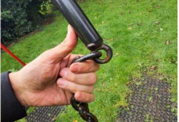
Finding: There is some notable evidence of wear to the anti Action: Monitor for any further deterioration and replace when 40% worn
