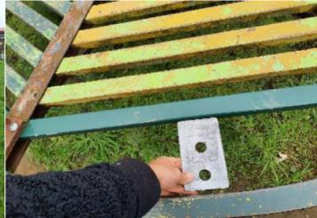
Finding: The item fails to meet the requirements of BS EN Action: Monitor - No remedial work recommended 1176 Part 1 4.2.7.2 for head and neck entrapment in the framework
